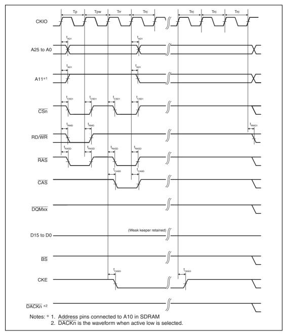
Figure 25.31 Synchronous DRAM Self-Refreshing Timing (WTRP = 1 Cycle)
