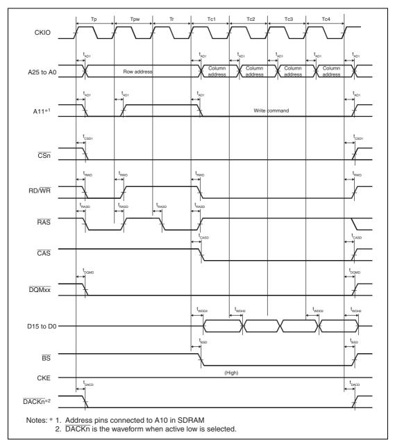
Figure 25.29 Synchronous DRAM Burst Write Bus Cycle (Single Write × 4)
