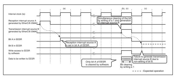
Figure 12.8 Timing of the Case where Setting of the Interrupt Source Bit in EESR by the E-DMAC Fails
