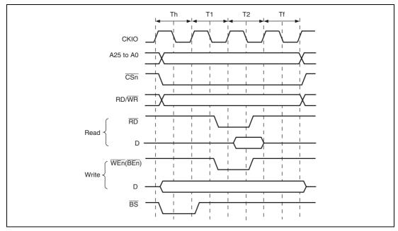
Figure 7.11 Example of Timing when CSn Assertion Period is Extended
