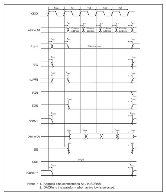
Figure 25.28 Synchronous DRAM Burst Write Bus Cycle (Single Write  $\times$  4) (Bank Active Mode: WRITE Command, Same Row Address, WTRCD = 0 Cycle, TRWL = 0 Cycle)
