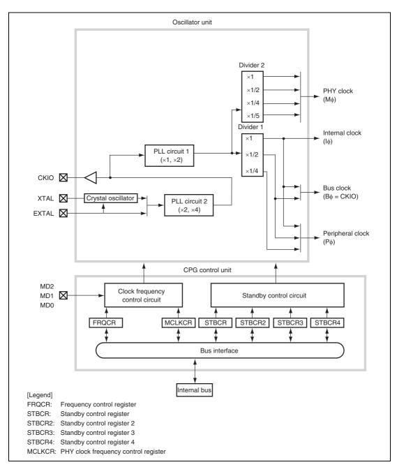
Figure 8.1 Block Diagram of CPG
