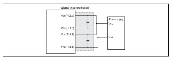
Figure 8.3 Note on Using a PLL Oscillator Circuit
