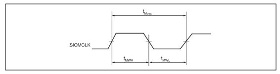
Figure 25.41 SIOMCLK Input Timing
