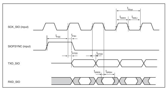
Figure 25.46 SIOF Transmit/Receive Timing (Slave Mode 1/ Slave Mode 2)
