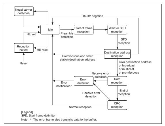
Figure 11.3 EtherC Receiver State Transmissions
