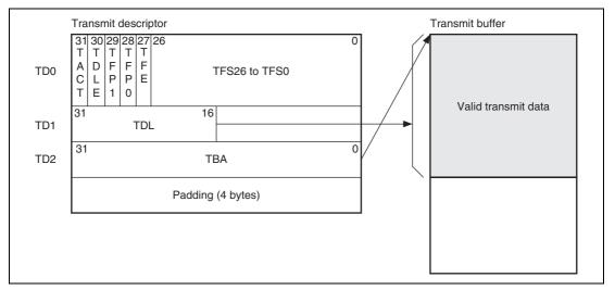
Figure 12.2 Relationship between Transmit Descriptor and Transmit Buffer
