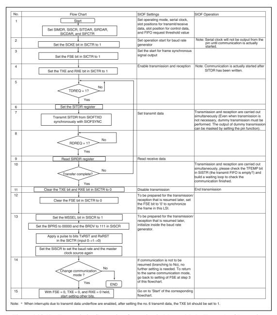
Figure 16.9 (1) Transmission/Reception Operation in Master Mode (Example of Reception and Full-Duplex Transmission by the CPU with TDMAE=0)
