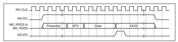
Figure 11.4 (5) MII Frame Receive Timing (Reception Error (1))
