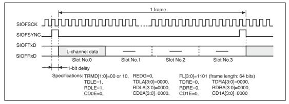
Figure 16.15 Transmit and Receive Timing (16-Bit Monaural Data (1))
