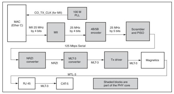
Figure 22.6 100Base-TX Data Path
