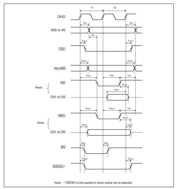
Figure 25.10 Basic Bus Timing: No Wait Cycle
