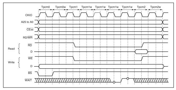
Figure 7.35 Wait Timing for PCMCIA Memory Card Interface (TED[3:0] = B'0010, TEH[3:0] = B'0001, Software Wait = 1, Hardware Wait = 1)
