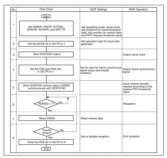
Figure 16.10 Example of Receive Operation in Master Mode
