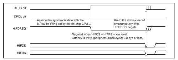
Figure 17.8 HIFDREQ Timing (When DMD = 0 and DPOL = 0)
