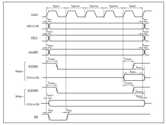
Figure 25.35 PCMCIA I/O Card Interface Bus Timing
