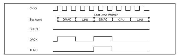
Figure 13.17 Example of DMA Transfer End in Cycle Steal Mode Level Detection
