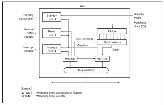
Figure 9.1 Block Diagram of WDT
