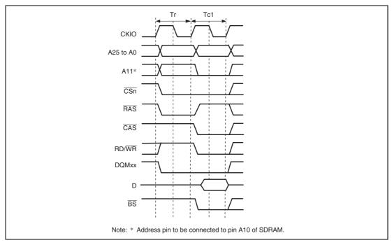
Figure 7.22 Single Write Timing (No Auto Precharge)
