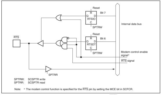
Figure 15.19 RTSIO Bit, RTSDT Bit, and RTS Pin
