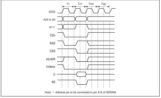
Figure 7.18 Basic Timing for Single Write (Auto-Precharge)
