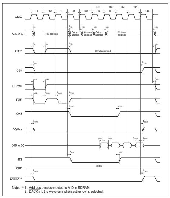
Figure 25.26 Synchronous DRAM Burst Read Bus Cycle (Single Read × 4)
