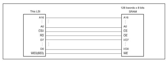
Figure 7.8 Example of 8-Bit Data-Width SRAM Connection
