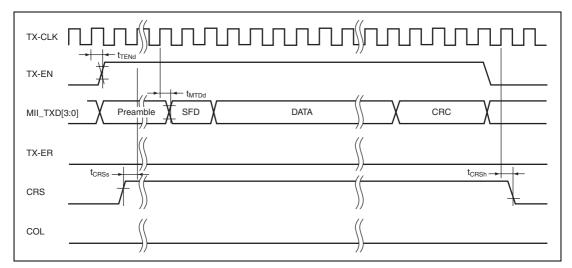
Figure 25.51 MII Transmission Timing (Normal Operation)
