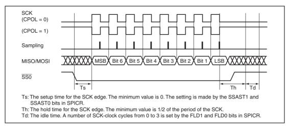
Figure 16.23 SPI Data/Clock Timing 2 (CPHA = 1)
