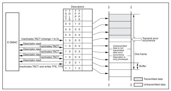
Figure 12.6 E-DMAC Operation after Transmit Error
