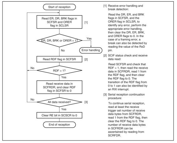
Figure 15.7 Sample Flowchart for Receiving Serial Data (1)
