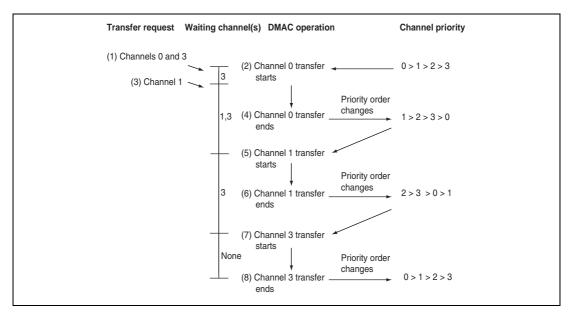
Figure 13.4 Changes in Channel Priority in Round-Robin Mode
