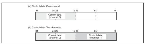
Figure 16.6 Control Data Bit Alignment
