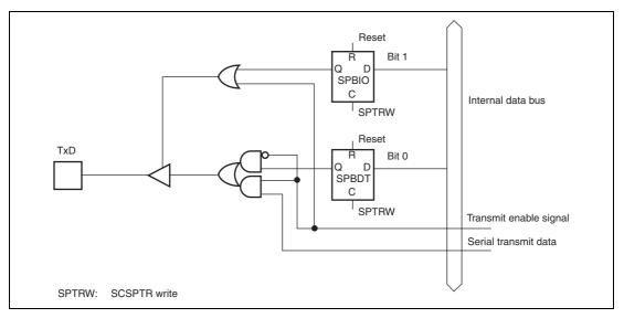
Figure 15.22 SPBIO Bit, SPBDT Bit, and TxD Pin
