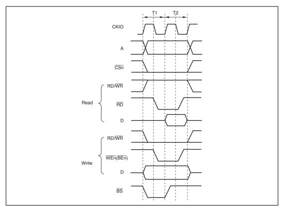
Figure 7.3 Normal Space Basic Access Timing (No-Wait Access)
