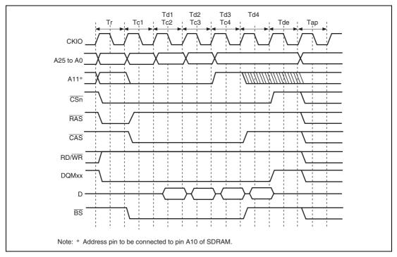
Figure 7.14 Burst Read Basic Timing (Auto Precharge)
