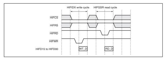
Figure 17.4 HIFIDX Write and HIFGSR Read
