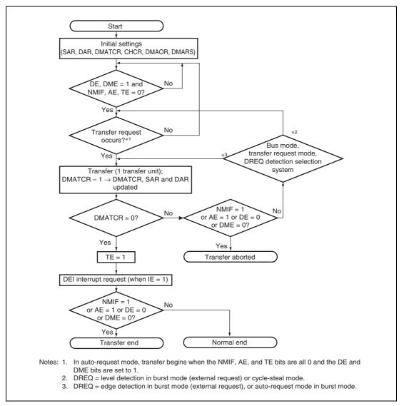
Figure 13.2 DMA Transfer Flowchart
