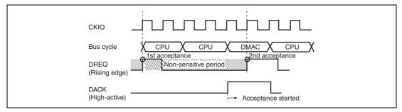
Figure 13.13 Example of DREQ Input Detection in Cycle Steal Mode Edge Detection
