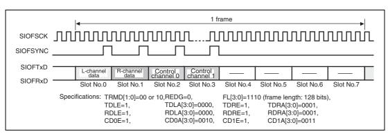
Figure 16.20 Transmit and Receive Timing (16-Bit Stereo Data)
