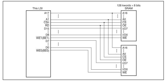
Figure 7.7 Example of 16-Bit Data-Width SRAM Connection
