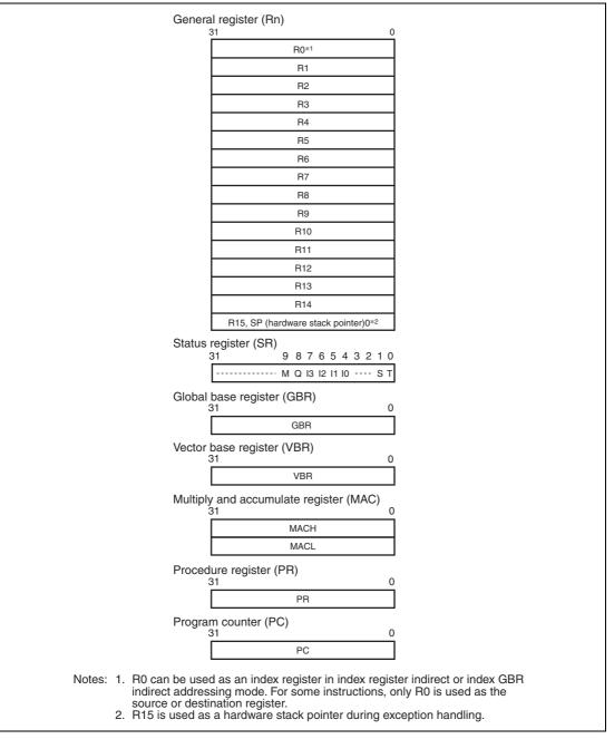
Figure 2.1 CPU Internal Register Configuration
