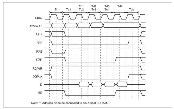
Figure 7.19 Burst Read Timing (No Auto Precharge)
