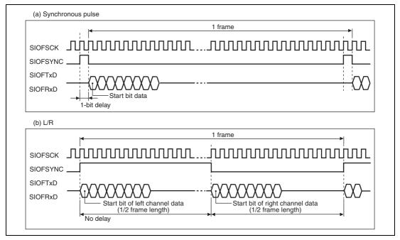
Figure 16.3 Serial Data Synchronization Timing
