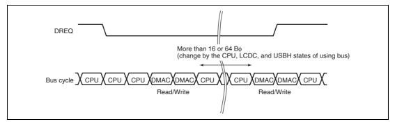
Figure 13.10 Example of DMA Transfer in Cycle Steal Intermittent Mode (Dual Address, DREQ Low Level Detection)
