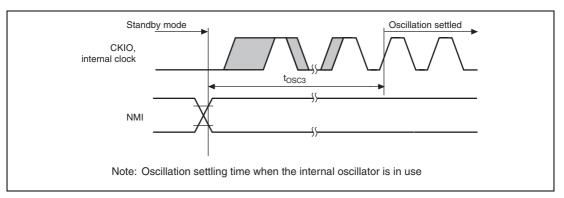
Figure 25.5 Oscillation Settling Timing after Standby Mode (By NMI or IRQ)
