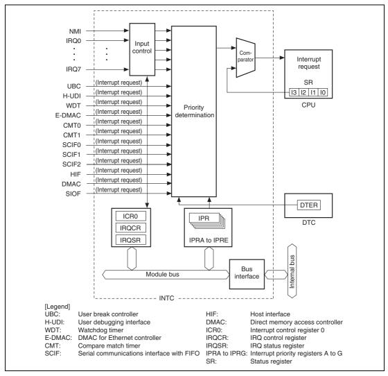
Figure 6.1 INTC Block Diagram
