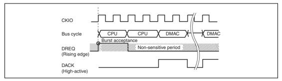
Figure 13.15 Example of DREQ Input Detection in Burst Mode Edge Detection
