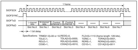
Figure 16.18 Transmit and Receive Timing (16-Bit Stereo Data (3))
