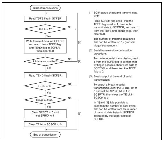
Figure 15.4 Sample Flowchart for Transmitting Serial Data
