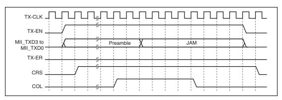
Figure 11.4 (2) MII Frame Transmit Timing (Collision)
