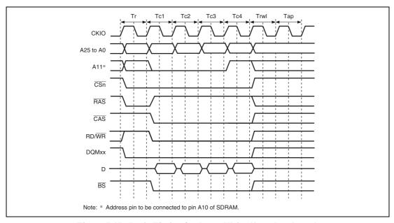
Figure 7.17 Basic Timing for Burst Write (Auto Precharge)
