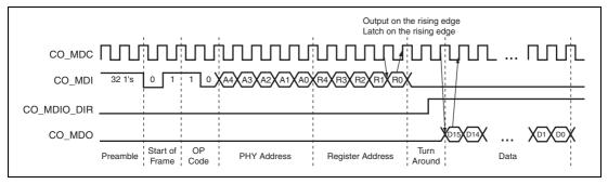
Figure 22.4 MDIO Timing and Frame Structure (READ Cycle)
