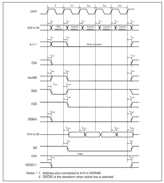
Figure 25.27 Synchronous DRAM Burst Write Bus Cycle (Single Write × 4)
