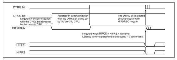
Figure 17.9 HIFDREQ Timing (When DMD = 0 and DPOL = 1)
