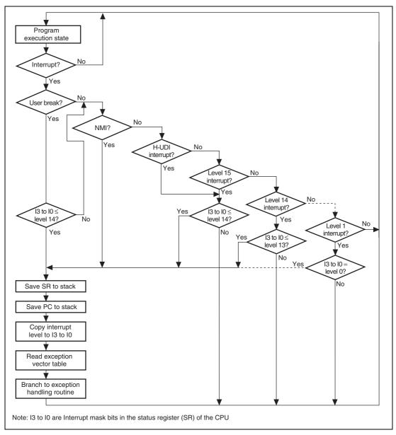
Figure 6.3 Interrupt Sequence Flowchart
