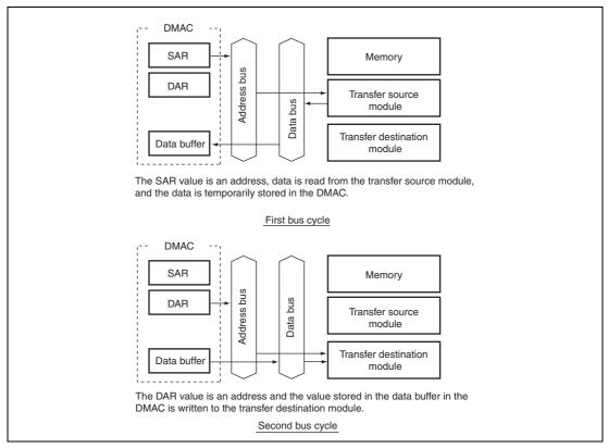
Figure 13.5 Data Flow of Dual Address Mode
