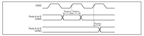
Figure 25.47 I/O Port Timing
