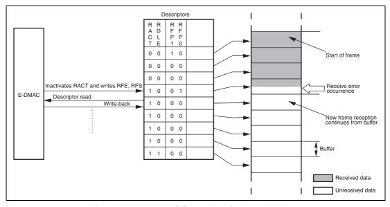
Figure 12.7 E-DMAC Operation after Receive Error
