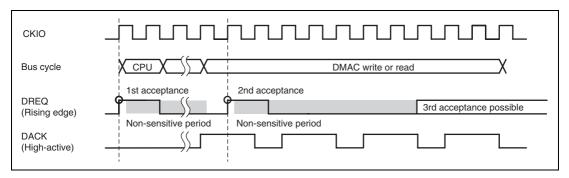
Figure 13.19 Example of DREQ Input Detection in Cycle Steal Mode Edge Detection When DACK is Divided to 4 by Idle Cycles
