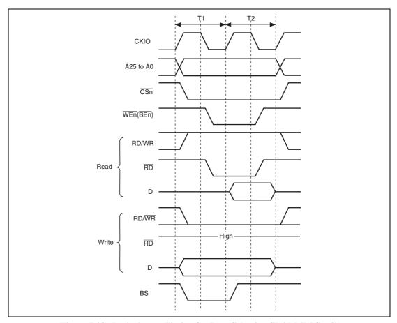
Figure 7.28 Basic Access Timing for Byte-Selection SRAM (BAS = 0)
