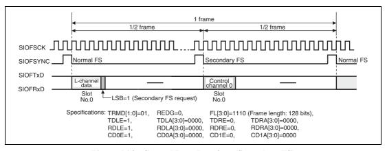
Figure 16.8 Control Data Interface (Secondary FS)
