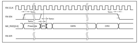
Figure 25.53 MII Reception Timing (Normal Operation)
