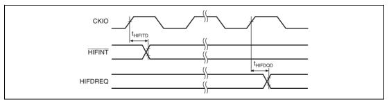
Figure 25.49 HIFINT and HIFDREQ Timing
