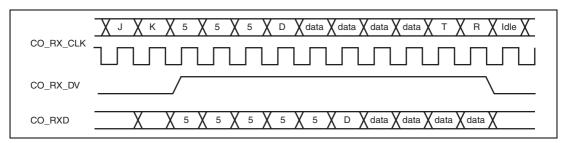
Figure 22.8 Relationship between Received Data and Some MII Signals
