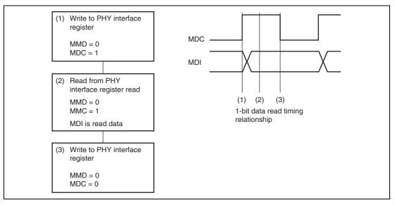
Figure 11.6 (3) 1-Bit Data Read Flowchart
