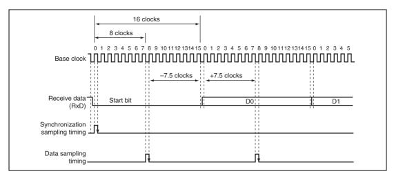
Figure 15.24 Receive Data Sampling Timing in Asynchronous Mode
