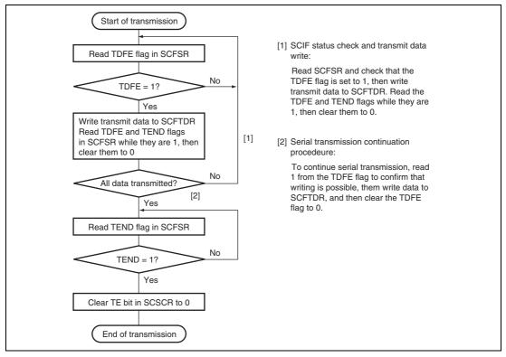
Figure 15.13 Sample Flowchart for Transmitting Serial Data
