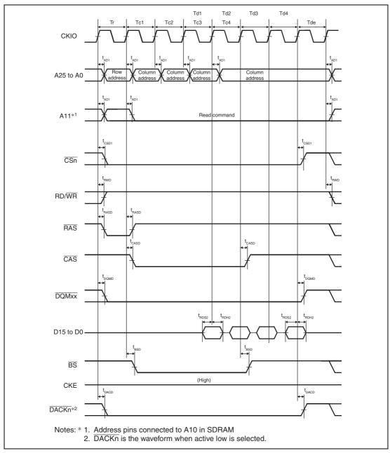
Figure 25.24 Synchronous DRAM Burst Read Bus Cycle (Single Read  $\times$  4) (Bank Active Mode: ACT + READ Commands, CAS Latency = 2, WTRCD = 0 Cycle)
