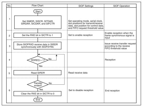
Figure 16.12 Example of Receive Operation in Slave Mode
