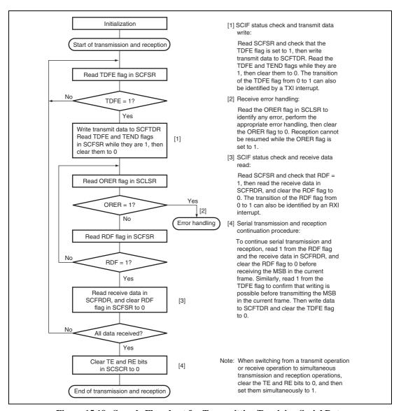
Figure 15.18 Sample Flowchart for Transmitting/Receiving Serial Data
