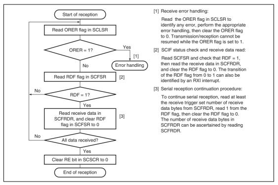
Figure 15.15 Sample Flowchart for Receiving Serial Data (1)
