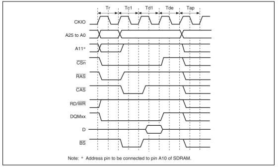
Figure 7.16 Basic Timing for Single Read (Auto Precharge)
