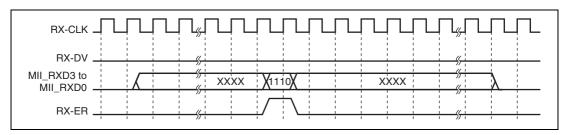
$Figure\ 11.4\ (6)\quad MII\ Fame\ Receive\ Timing\ (Reception\ Error\ (2))$
