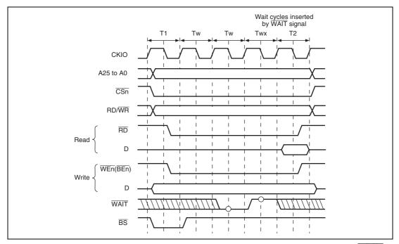
Figure 7.10 Wait Cycle Timing for Normal Space Access (Wait cycle Insertion using WAIT)
