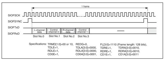
Figure 16.7 Control Data Interface (Slot Position)
