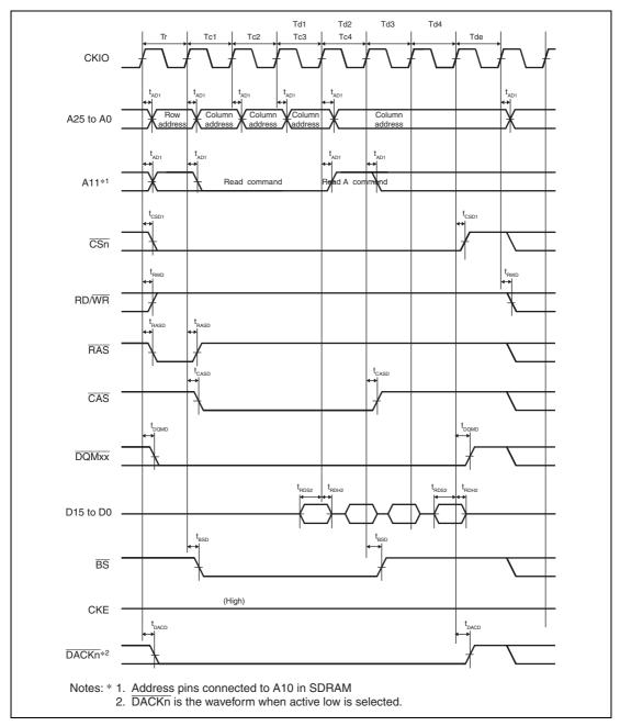
Figure 25.18 Synchronous DRAM Burst Read Bus Cycle (Single Read × 4) (Auto-Precharge, CAS Latency = 2, WTRCD = 0 Cycle, WTRP = 1 Cycle)
