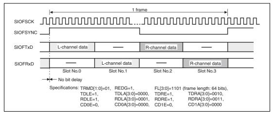
Figure 16.17 Transmit and Receive Timing (16-Bit Stereo Data (2))
