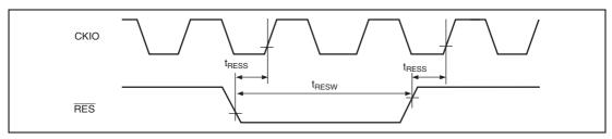
Figure 25.7 Reset Input Timing
