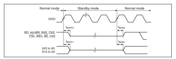
Figure 25.9 Pin Drive Timing in Standby Mode
