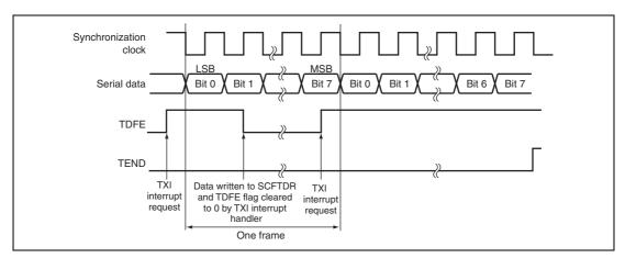
Figure 15.14 Example of SCIF Transmit Operation
