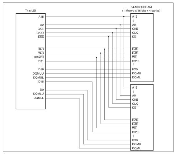
Figure 7.12 Example of 32-Bit Data-Width SDRAM Connection
