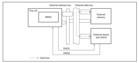
Figure 13.7 Data Flow in Single Address Mode
