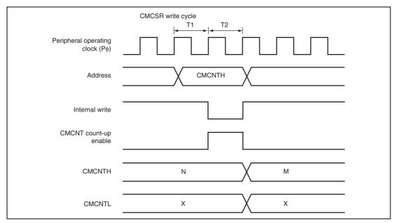
Figure 14.7 Conflict between Byte-Write and Count-Up Processes of CMCNT
