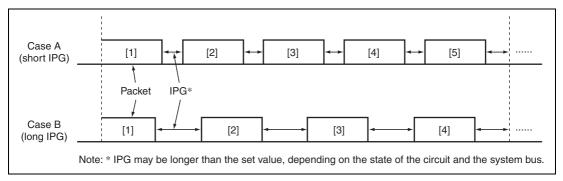
Figure 11.7 Changing IPG and Transmission Efficiency
