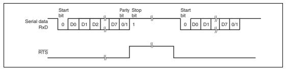
Figure 15.10 Example of Operation Using Modem Control (RTS)
