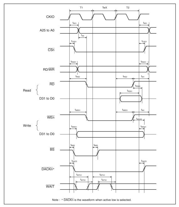
Figure 25.12 Basic Bus Timing: One External Wait Cycle
