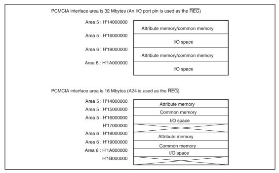
Figure 7.36 Example of PCMCIA Space Assignment (CS5BWCR.SA[1:0] = B'10, CS6BWCR.SA[1:0] = B'10)
