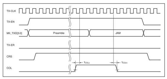
Figure 25.52 MII Transmission Timing (Collision Occurred)
