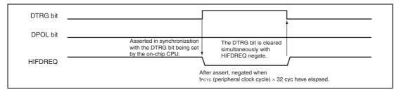
Figure 17.10 HIFDREQ Timing (When DMD = 1 and DPOL = 0)
