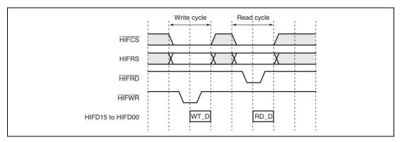
Figure 17.3 Basic Timing for HIF Interface
