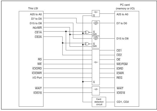
Figure 7.33 Example of PCMCIA Interface Connection
