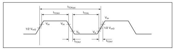
Figure 25.59 TCK Input Timing
