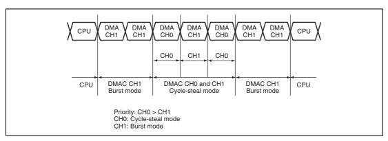
Figure 13.12 Bus State when Multiple Channels are Operating
