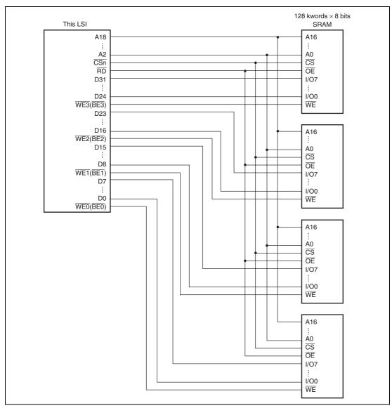
Figure 7.6 Example of 32-Bit Data-Width SRAM Connection
