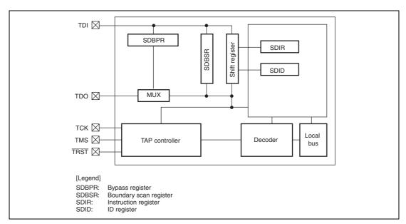
Figure 21.1 Block Diagram of H-UDI
