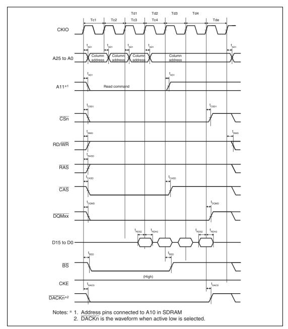
Figure 25.25 Synchronous DRAM Burst Read Bus Cycle (Single Read × 4) (Bank Active Mode: READ Command, Same Row Address, CAS Latency = 2, WTRCD = 0 Cycle)
