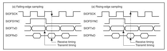
Figure 16.4 SIOF Transmit/Receive Timing
