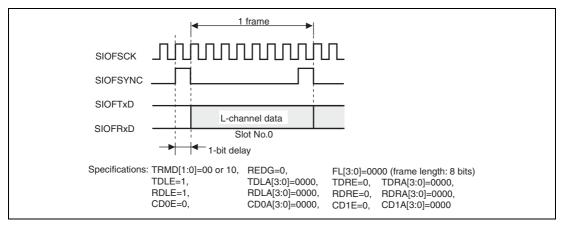
Figure 16.13 Transmit and Receive Timing (8-Bit Monaural Data (1))
