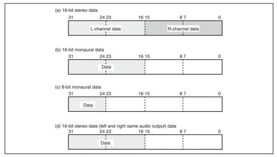
Figure 16.5 Transmit/Receive Data Bit Alignment
