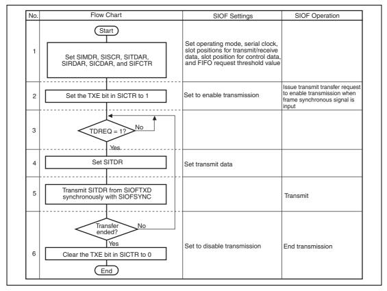
Figure 16.11 Example of Transmit Operation in Slave Mode
