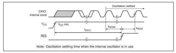
Figure 25.3 Oscillation Settling Timing after Power-On
