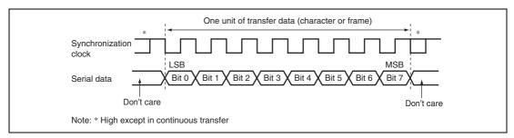
Figure 15.11 Data Format in Synchronous Communication
