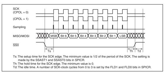
Figure 16.22 SPI Data/Clock Timing 1 (CPHA = 0)
