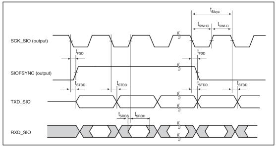
Figure 25.45 SIOF Transmit/Receive Timing (Master Mode 2/Rising Edge Sampling)
