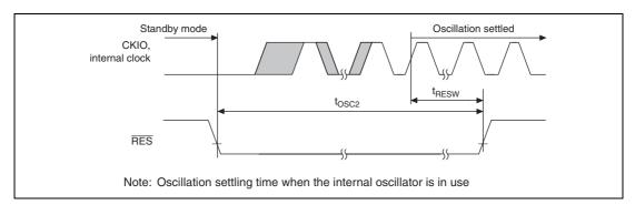
Figure 25.4 Oscillation Settling Timing after Standby Mode (By Reset)
