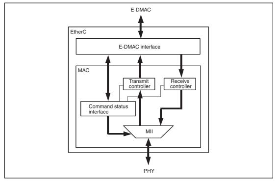
Figure 11.1 Configuration of EtherC
