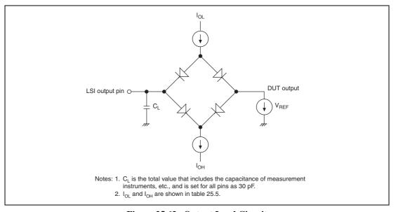
Figure 25.62 Output Load Circuit
