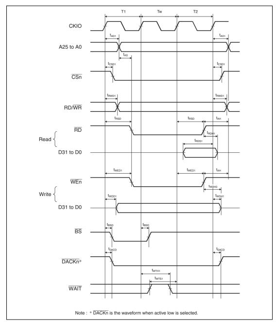
Figure 25.11 Basic Bus Timing: One Software Wait Cycle
