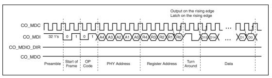
Figure 22.5 MDIO Timing and Frame Structure (WRITE Cycle)
