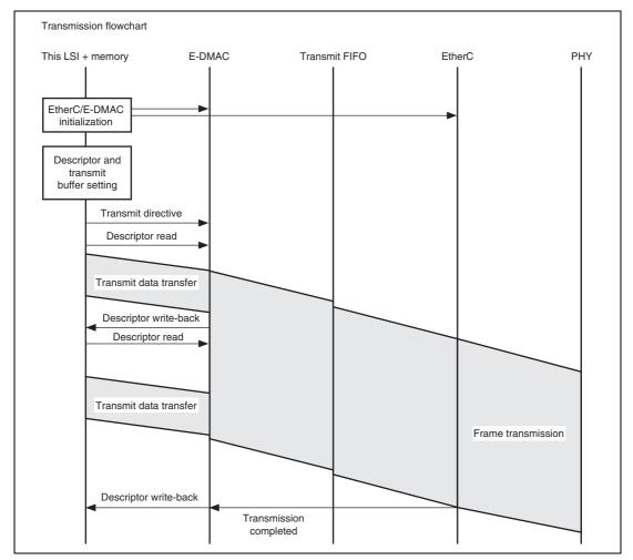
Figure 12.4 Sample Transmission Flowchart
