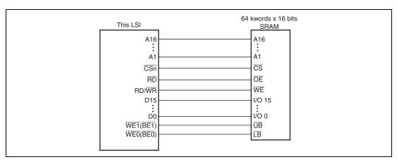
Figure 7.32 Example of Connection with 16-Bit Data-Width Byte-Selection SRAM
