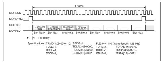
Figure 16.19 Transmit and Receive Timing (16-Bit Stereo Data (4))
