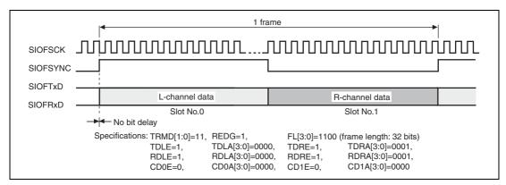
Figure 16.16 Transmit and Receive Timing (16-Bit Stereo Data (1))
