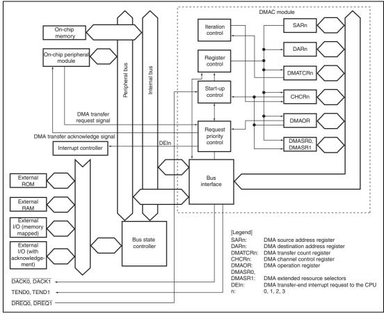
Figure 13.1 Block Diagram of DMAC
