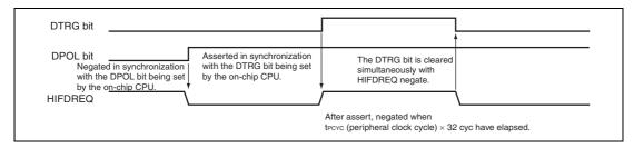
Figure 17.11 HIFDREQ Timing (When DMD = 1 and DPOL = 1)
