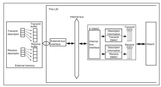
Figure 12.1 Configuration of E-DMAC, and Descriptors and Buffers
