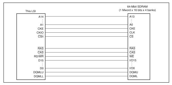
Figure 7.13 Example of 16-Bit Data-Width SDRAM Connection
