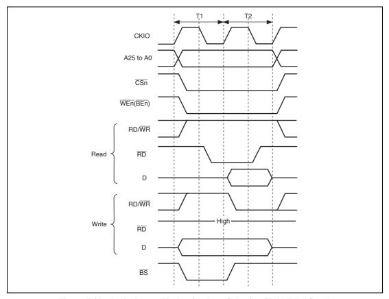
Figure 7.29 Basic Access Timing for Byte-Selection SRAM (BAS = 1)
