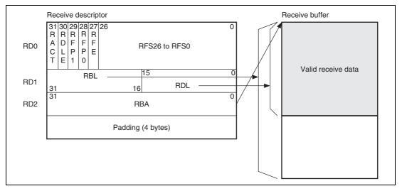
Figure 12.3 Relationship between Receive Descriptor and Receive Buffer
