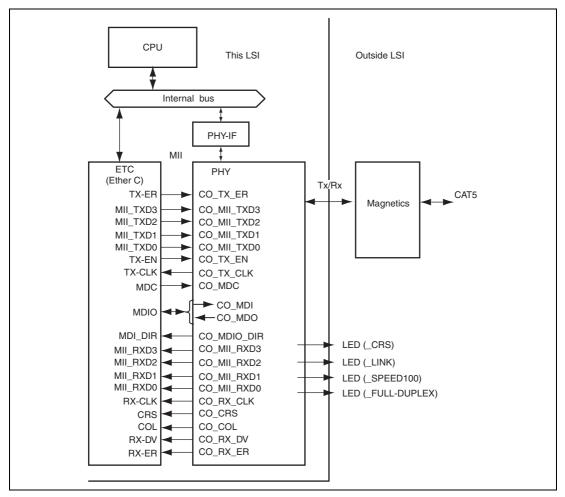
Figure 22.1 The Block Diagram around PHY Module
