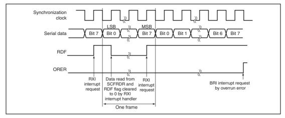
Figure 15.17 Example of SCIF Receive Operation
