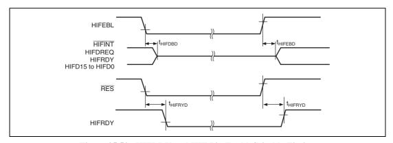
Figure 25.50 HIFRDY and HIF Pin Enable/Disable Timing
