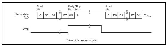
Figure 15.6 Example of Operation Using Modem Control (CTS)
