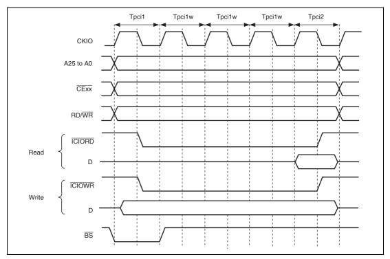
Figure 7.37 Basic Timing for PCMCIA I/O Card Interface
