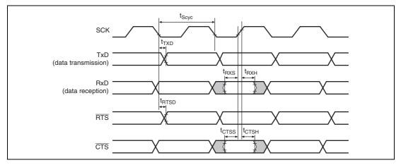
Figure 25.40 SCI Input/Output Timing in Clocked Synchronous Mode
