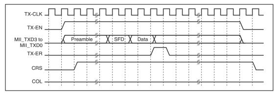
**Figure 11.4 (3) MII Frame Transmit Timing (Transmit Error)**
