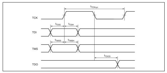
Figure 25.61 H-UDI Data Transmission Timing
