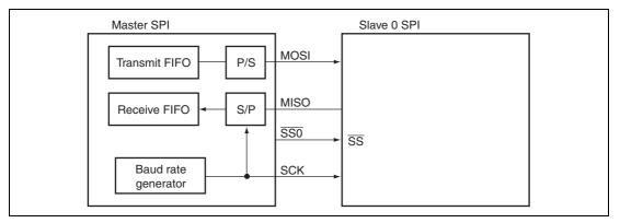
Figure 16.21 Example of Configuration in SPI Mode
