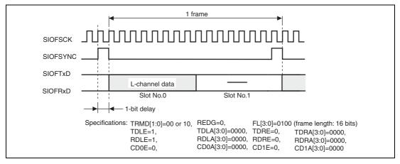
Figure 16.14 Transmit and Receive Timing (8-Bit Monaural Data (2))
