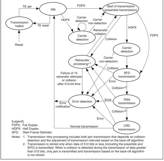
Figure 11.2 EtherC Transmitter State Transitions
