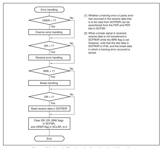
Figure 15.8 Sample Flowchart for Receiving Serial Data (2)
