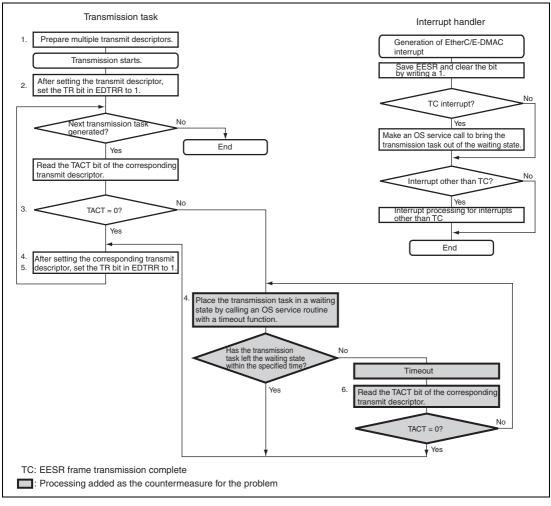
Figure 12.10 Method of Adding Timeout Processing
