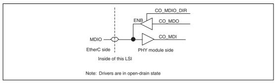
Figure 22.3 How to Derive MDIO Signal from Core Signals
