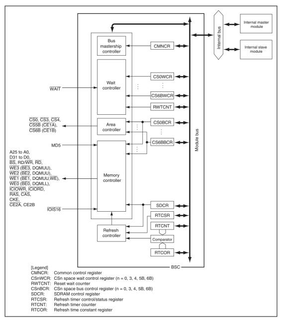
Figure 7.1 Block Diagram of BSC
