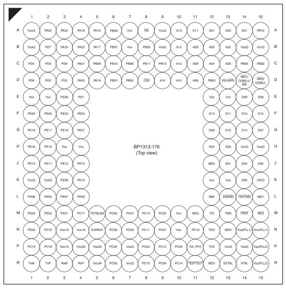
Figure 1.2 Pin Assignments
