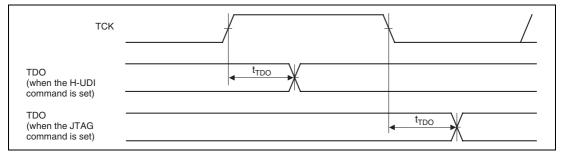
Figure 21.3 H-UDI Data Transfer Timing
