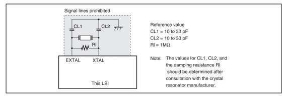
Figure 8.2 Note on Using a Crystal Resonator
