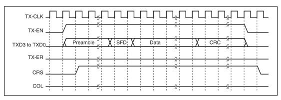
Figure 11.4 (1) MII Frame Transmit Timing (Normal Transmission)
