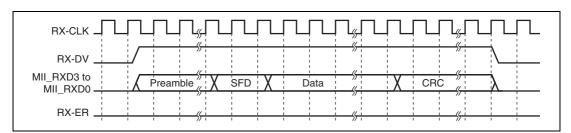
Figure 11.4 (4) MII Frame Receive Timing (Normal Reception)
