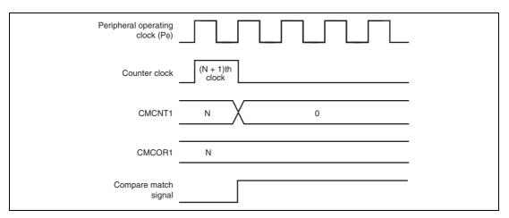
Figure 14.4 Timing of CMF Setting
