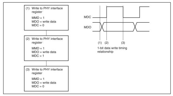
Figure 11.6 (1) 1-Bit Data Write Flowchart
