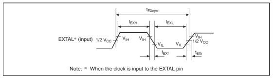
Figure 25.1 External Clock Input Timing
