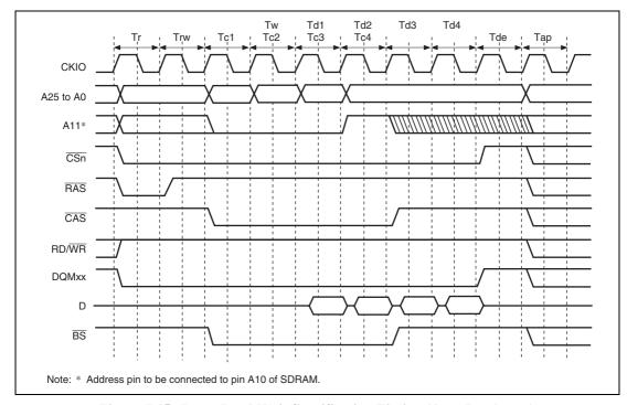
Figure 7.15 Burst Read Wait Specification Timing (Auto Precharge)
