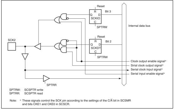
Figure 15.21 SCKIO Bit, SCKDT Bit, and SCK Pin
