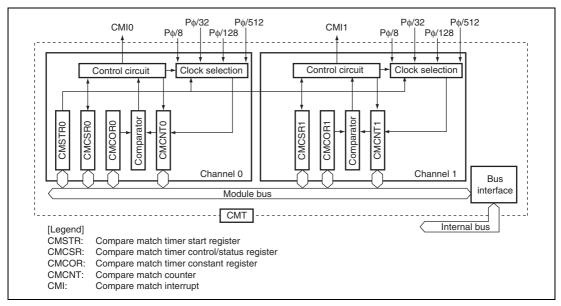
Figure 14.1 Block Diagram of Compare Match Timer
