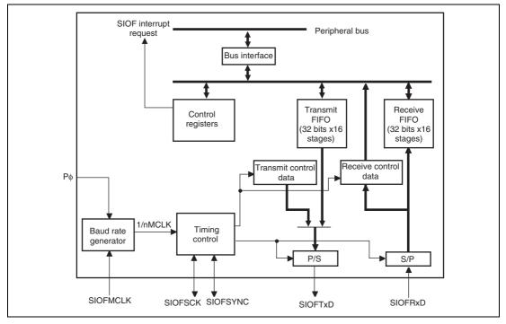
Figure 16.1 Block Diagram of SIOF
