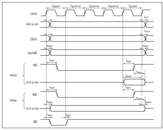
Figure 25.33 PCMCIA Memory Card Interface Bus Timing
