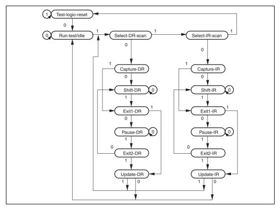
Figure 21.2 TAP Controller State Transitions
