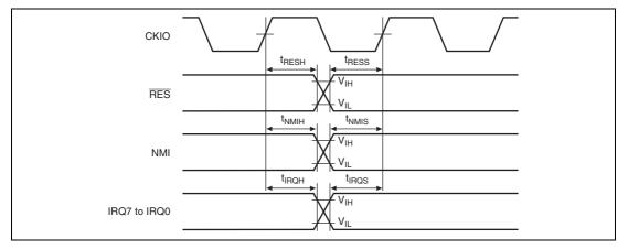
Figure 25.8 Interrupt Input Timing
