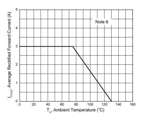
Figure 1. Forward Current Derating Curve
