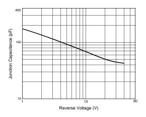
Figure 5. Typical Junction Capacitance
