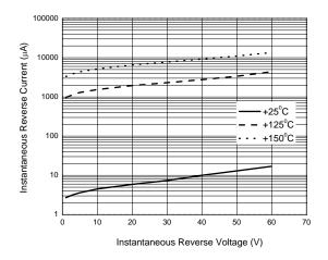
Figure 4. Typical Reverse Characteristics
