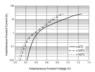
Figure 2. Typical Instantaneous Forward Characteristics
