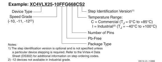
Figure 1: Virtex-4 FPGA Ordering Information
