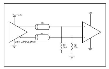
Figure 2C. 2.5V LVPECL Driver Termination Example
