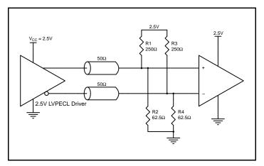
Figure 2A. 2.5V LVPECL Driver Termination Example
