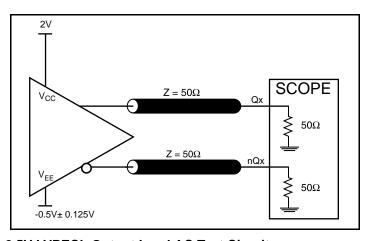
2.5V LVPECL Output Load AC Test Circuit
