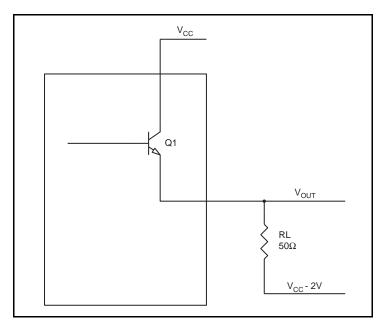
Figure 4. LVPECL Driver Circuit and Termination
