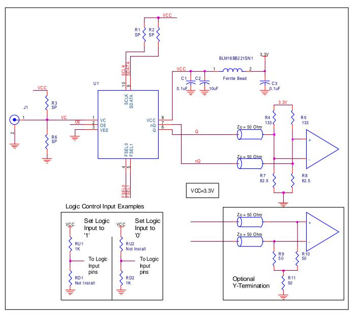
Figure 3. IDT8N3QV01 Application Schematic
