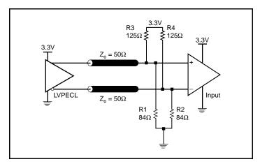
Figure 1B. 3.3V LVPECL Output Termination
