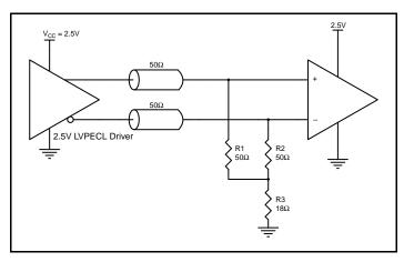
Figure 2B. 2.5V LVPECL Driver Termination Example
