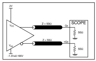
3.3V LVPECL Output Load AC Test Circuit
