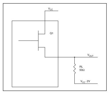
Figure 4. LVPECL Driver Circuit and Termination
