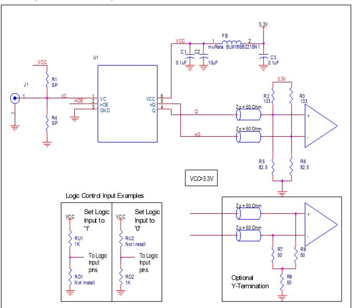
Figure 3. IDT8N3SV76 Application Schematic
