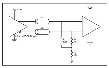
Figure 2B. 2.5V LVPECL Driver Termination Example
