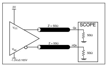
3.3V LVPECL Output Load AC Test Circuit
