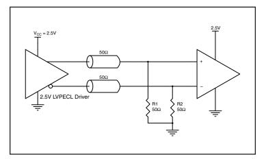
Figure 2C. 2.5V LVPECL Driver Termination Example
