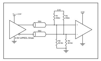
Figure 2A. 2.5V LVPECL Driver Termination Example
