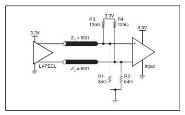
Figure 1B. 3.3V LVPECL Output Termination
