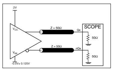
2.5V LVPECL Output Load AC Test Circuit
