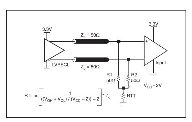
Figure 1A. 3.3V LVPECL Output Termination
