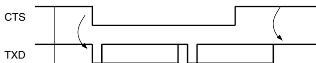
Figure 31-21. Transmitter Behavior when Operating with Hardware Handshaking
